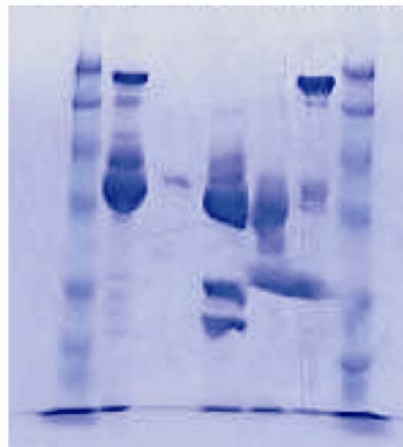
Figure 6: Purity of antibody separated on Toyopearl Phenyl-650M SDS gel of collected fractions. Fraction 4 shows very good purity of the Anti-TSH antibody
