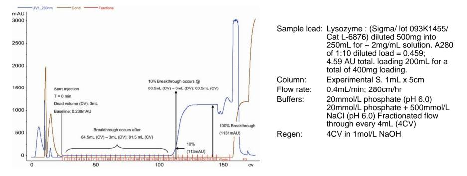
Based on simple overlays of both chromatography runs at 50 cycles and fresh resin, breakthrough occurs approximately at the same volume loading at 2mg/mL. Exposure time was 1h in 1mol/L NaOH for each cycle. Caustic stability data shows that the Experimental S resin stands up to multiple cleanings with no measurable loss in binding capacity.
