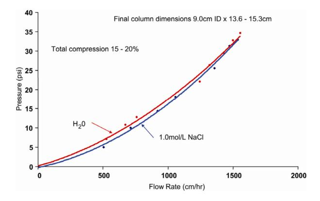
The experimental S resin was packed into a 9cm Millipore column to measure the pressure/flow characteristics. The resin had similar profiles for both water and 1.0mol/L NaCl.
