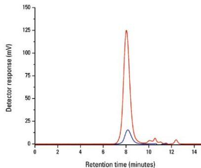
Figure 8. GPC elution profile of homopolymer, poly(1-hexene), as monitored by the RI
