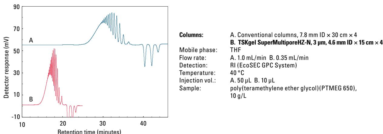
A comparison of chromatograms obtained from conventional and semi-micro TSKgel HxL and SuperHZ series columns are shown in **Figures 15 and 16**. TSKgel HxL and SuperHZ series columns have similar separation performance, solvent compatibility, stationary phase composition, and column efficiency. The differences between the two column series are particle size and column length.
