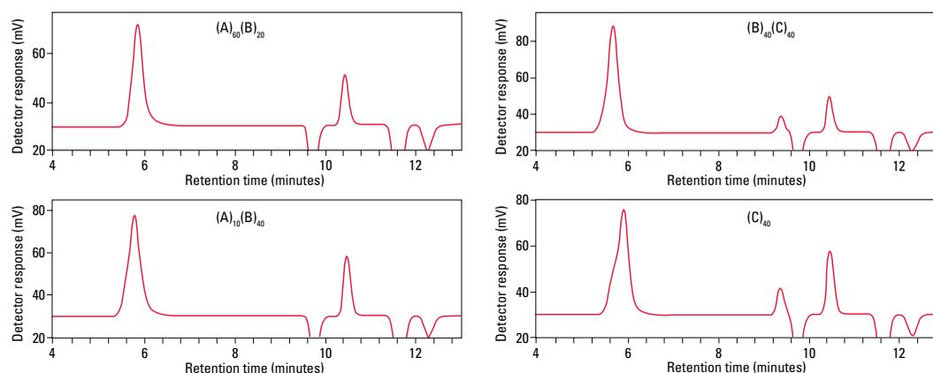
**Column:** TSKgel GMHHR-M, 5  $\mu$ m, 4.6 mm ID  $\times$  15 cm  $\times$  2 packed in HFIP
