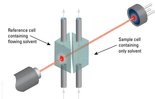
Figure 3: Depiction of RI detector flow cell showing the effects of THF degradation in the stagnant reference side of a conventional GPC system
