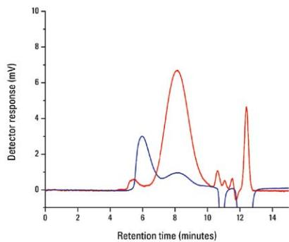
Figure 7. GPC elution profile of homopolymer, poly(3-hexylthiophene), as monitored by the RI (blue) and UV (red)
