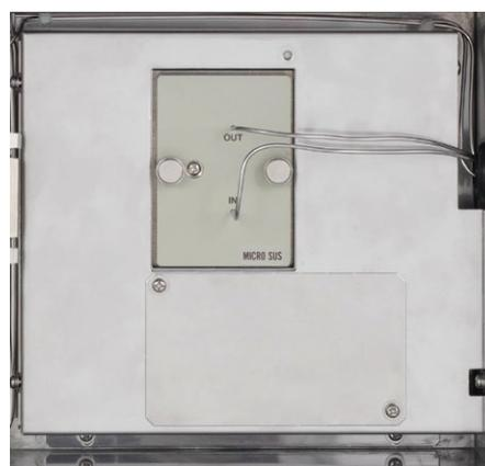
The optional UV detector is variable from 195 to 350 nm and the detector flow path and electronics are optimized for the use of semi-micro columns. The volume of the flow cell is reduced to 2  $\mu$ L and the shortest time constant is 0.5 seconds.
