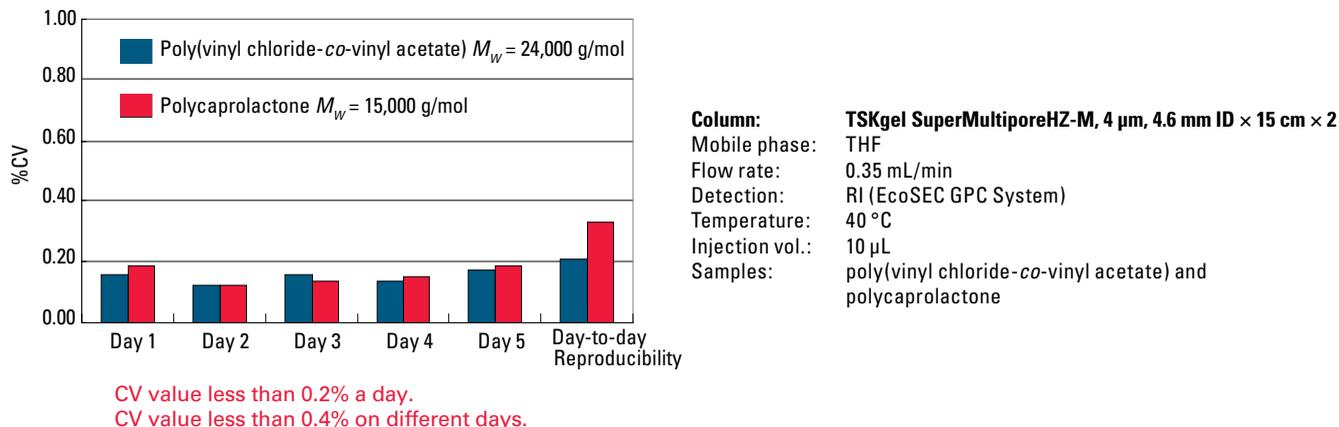
Figure 10 shows a comparison of  $M_w$  reproducibility for a sample injected 10 times a day for 5 days on the EcoSEC GPC System compared to a conventional GPC system. The reproducibility of the EcoSEC GPC System was superior by a factor of 3 to that of the conventional GPC system.
