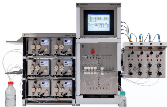
Figure 2. Bench-top Octave BIO MCC instrument with SkillPak™ BIO columns.
