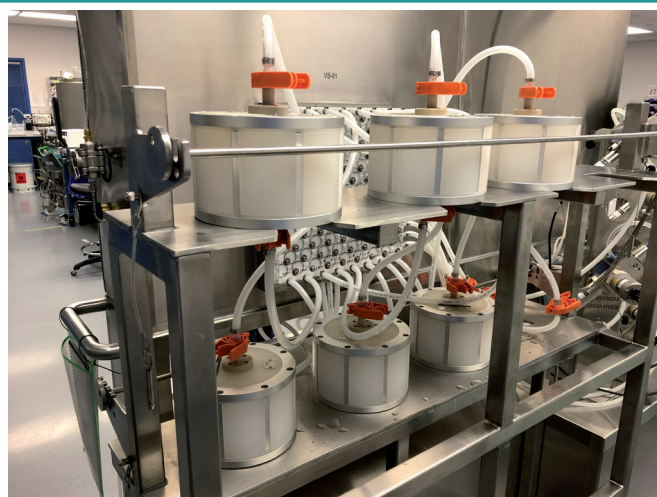
➤ Figure 3. The SkillPak PRO columns installed for the scaled-up MCC process.
