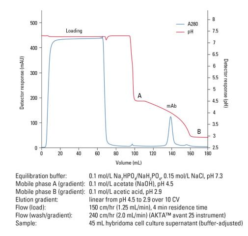
A sharp mAb peak with elution max at pH 4.0 was obtained using a linear pH gradient.
