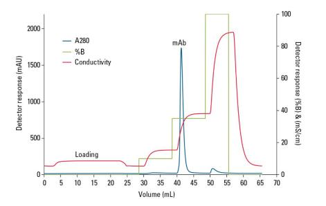
Equilibration buffer: 0.1 mol/L acetate (NaOH), pH 5.0 Post-loading 1st wash: equilibration buffer (5 CV) Post-loading 2nd wash: 0.1 mol/L acetate (NaOH), 0.1 mol/L NaCl, pH 5.0 (10 CV) 0.1 mol/L acetate (NaOH), 0.35 mol/L NaCl, pH 5.0 (10 CV) Elution: Column strip: 0.1 mol/L acetate (NaOH), 1.0 mol/L NaCl, pH 5.0 (7 CV) Flow (all steps): 156 cm/hr (1.0 mL/min) (AKTA avant 25 instrument) Sample: 21 mL diluted protein A eluate Temperature: ambient (room temperature)
